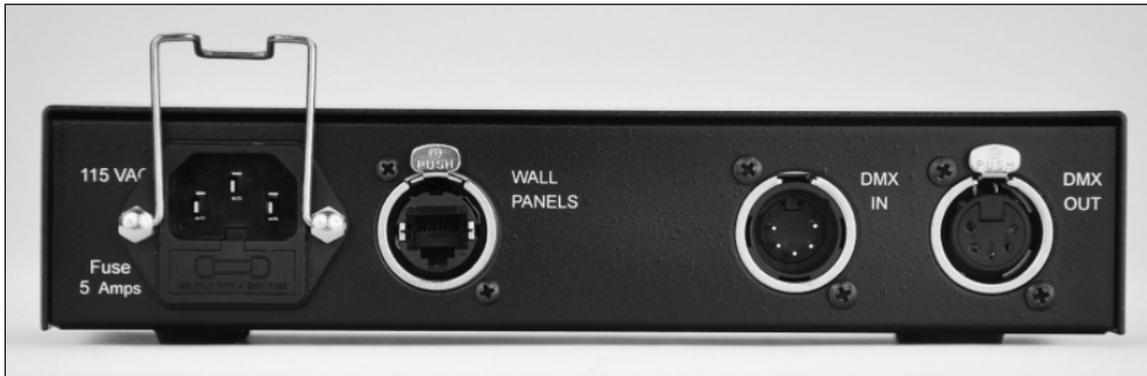
1. AC Power Input - IEC inlet with 5 amp fuse. A spare fuse is included in the fuse drawer in the lower part of the outlet. A locking wire bail can be used to secure the power cord.
