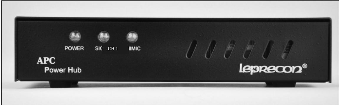
**Power** - this LED is lighted if the internal power supply is working properly.
