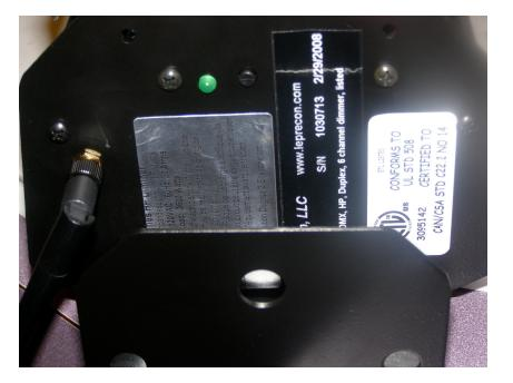
The LED located on the dimmer endplate shows the status of the wireless link.
