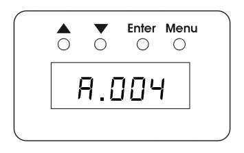
When valid DMX is detected, the letter 'A' is replaced with the letter 'd' for DMX:
