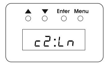
Set the mode for the displayed channel by pressing the UP/DOWN keys. The possible channel modes are:
