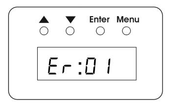
Error 01 is displayed for an overtemperature condition. Error 02 is displayed for an overvoltage condition.
