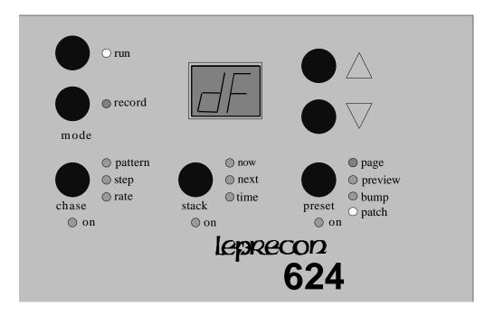
The **dF** display indicates the default, or straight 1:1 patch is in effect. To switch the board to the custom patch, press the up arrow next to the display.
