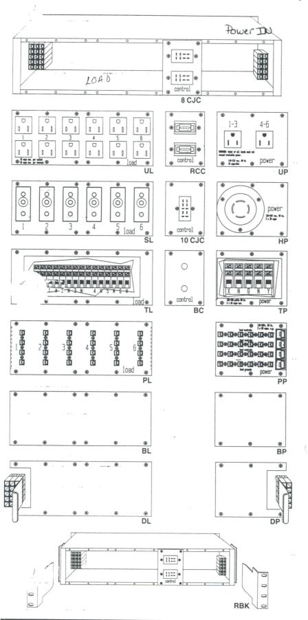
Load Panel Options Each dimmer has a 14 contact Amp Powerlock connector mounted internally. Load panels simply plug into this connector from the rear.
