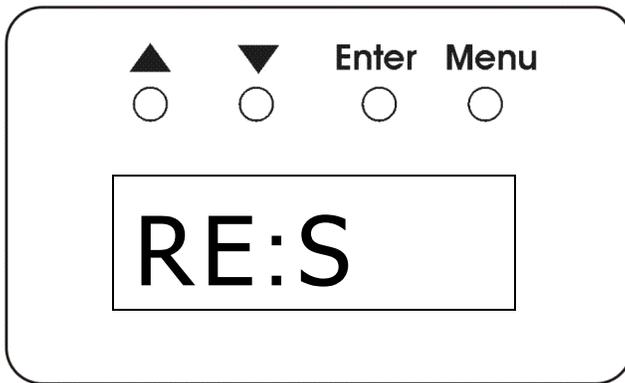
To reset the LDS dimmer, press and hold the Enter button. The colon will begin to flash. After about 5 seconds, the flashing will stop, and the dimmer will reset to Address mode.
