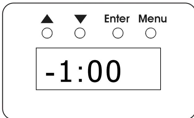
Once the input levels for all dimmer channels have been shown, the display will then indicate the output level for each channel. This is indicated by the letter 'o' in the display, followed by channel number, followed by output level. Output will be shown as a percentage, with 100% indicated by the letters 'FF'
