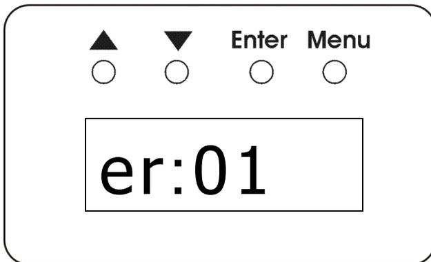
Error 01 is displayed for an over-temperature condition.
