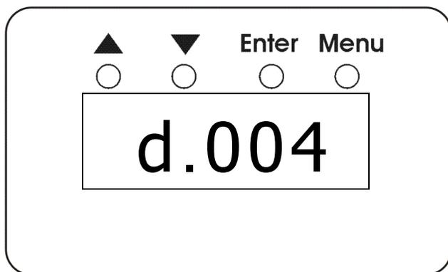
The UP/DOWN keys change the value for the start address. The LDS-610 uses the changed value immediately and permanently saves it after 10 seconds or if the Enter or Menu key is pressed.
