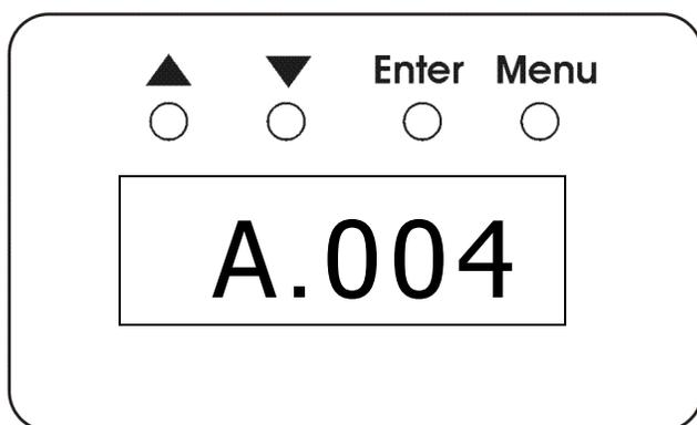
When valid DMX is detected, the letter 'A' is replaced with the letter 'd' for DMX:
