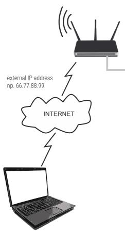
Router IP: 192.168.1.1 Mask: 255.255.255.0 DHCP: Off Redirecting port 50000 and 50001 to the device address (192.168.1.10)
