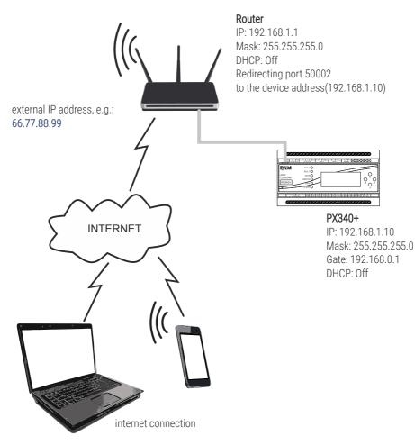
**NOTE!** If there are two controllers in network, the first one should be forwarded to the port 50002 and the second to e.g 60002 (the destination port is always port 50002).
