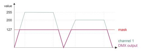
• minimal – it changes all the values in the channel that are smaller than the values of the mask to the values of the mask
