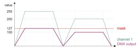
• maximal – it converts all the values in the channel that are greater than the value of the mask to the value of the mask
