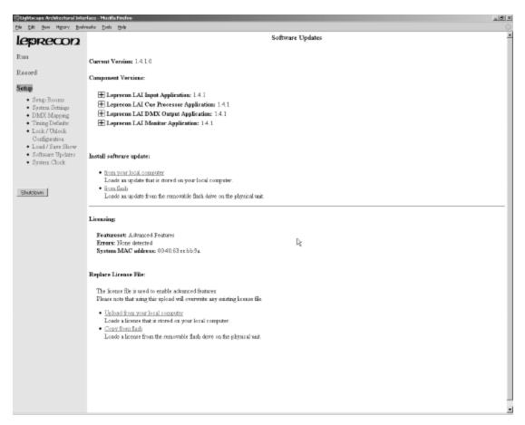
The software update screen displays current version information for all of the AI software applications. The interface will load new operating software from one of two sources, either the hard drive of your computer, or a USB Flash memory device.
