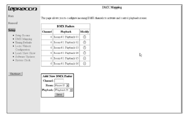
The table at the top of the screen shows current mapping; which incoming DMX channels can control specific playbacks. Click on the red X at the end of the line to delete a specific assignment.
