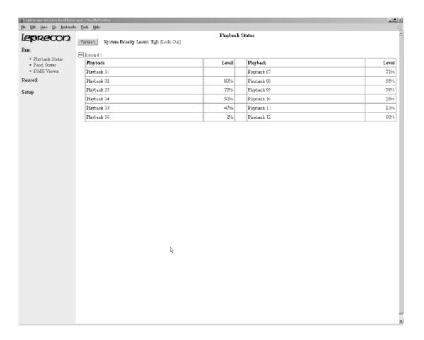
If multiple rooms are set up in the system, status is shown for each room. Each of the twenty eight playbacks are listed, and the output level of each playback is shown.
