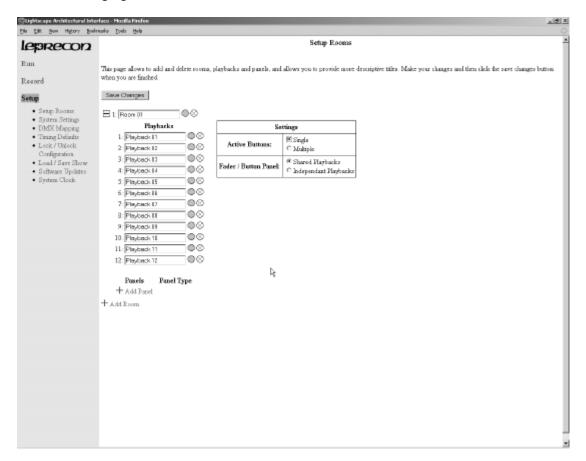
Using the AI-512 software, you can create and name playbacks and panels, even if the panels are not yet connected to the AI controller. Clicking on the 'Add Panel' or 'Add Room' menu items will create a new entry. Clicking on the red X at the end of the line will delete the room or panel.
