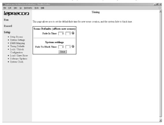
'Scene default' fade time is applied to all new scenes. The scene timing can be adjusted for each scene to a different value in the Record screen.
