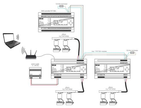
**NOTE!** A terminator – a 120  $\Omega$  resistor should be connected to the first (PX710M+) and the last (PX710S+) device.
